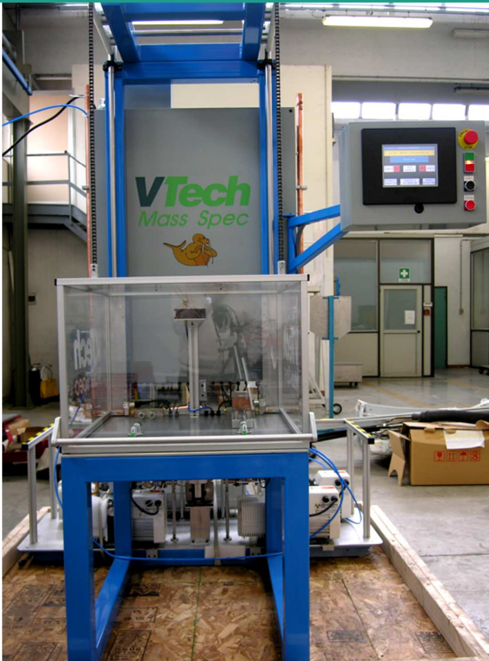
VTech MasSpec as installed at a major coil manufacturer in Asia, testing plate heat exchangers with internal circuit testing. Cycle time: 1 min for two coils.
